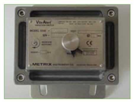
The switch **detects excessive fan drive vibration** caused by fan icing or any mechanical fault. Although factory mounted, the switch point is adjusted on-site during installation and start-up.
