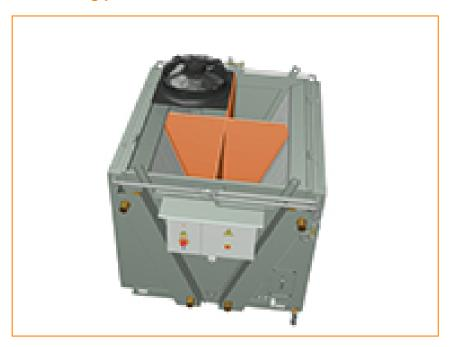
Equipping a unit with partition panels provides an **individual air intake duct for each and every fan** on the adiabatic cooler. This guarantees a higher capacity in case of fan failure by avoiding unintended air flows through an idle fan which bypasses the coil.
