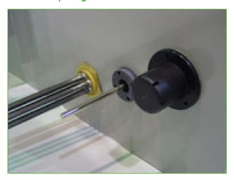
Our factory-installed heaters keep the water temperature at 4°C and act as a simple and economical **anti-freeze measure for the basin water** during shutdown or standby periods. The heater package includes the **heaters**, a **thermostat** and a **low level cut out switch** to protect the heaters if the water level declines excessively. Standard electric heaters can handle ambient temperatures down to -18°C.
