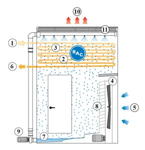
Refrigerant vapour (1) circulates through an evaporative condensing coil (2), which is continuously wetted by the spray system (3) installed at the top of the condenser. At the same time the individual driven axial fans (4), located at the bottom of the unit, blow ambient air (5) upwards through the condenser.
