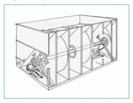
The installation of a Baltiquard® Drive System
