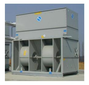
**If VX units are installed on a steel structure above ground level** several precautions must be considered. If the unit is installed more than 300mm above surface it is necessary for safety reasons to install a solid bottom panel to provide protection from moving parts ( sheaves, belts, motors, fan wheels, shafts,...).
