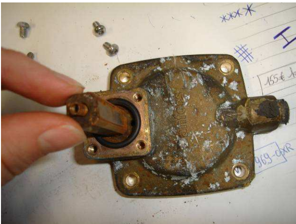
Remove screws to open valve
