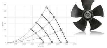
*Example:* Fan manufacturer indicates 85dB(A) sound power level for the fan in our operating point.
