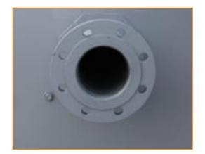
Flanges facilitate piping connections on-site.
