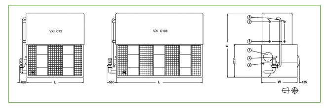
1. Drain ND xx; 2. Outlet connection NDxx; 3. Overflow NDxx; 4. Make up ND xx; 5. Inlet connection NDxx; 6. Vent NDxx; 7. Access door.
