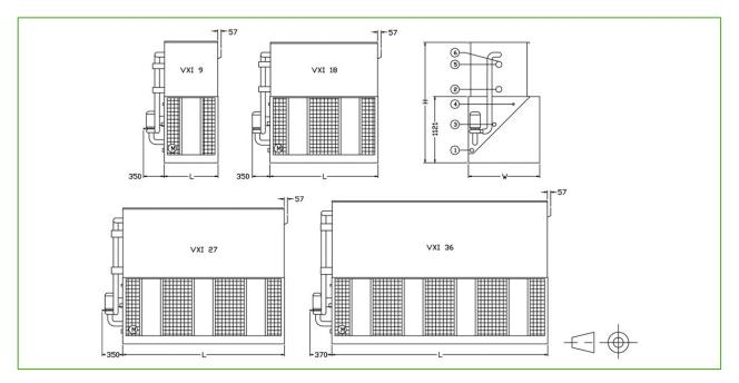
1. Drain ND50; 2. Outlet connection ND80 for VXI 9-X and ND100 for VXI 18-X, 27-X and 36-X; 3. Overflow ND50; 4. Make up ND25; 5. Inlet connection ND80 for VXI 9-X and ND100 for VXI 18-X, 27-X and 36-X; 6. Vent ND15; 7. Access door (not shown).
