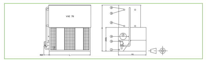
1. Drain ND50; 2. Outlet connection ND100; 3. Overflow ND80; 4. Make up ND50; Inlet connection ND100; 6. Vent ND15; 7. Access door.
