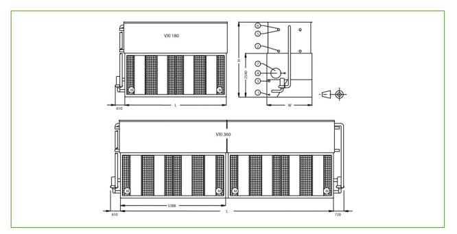
1. Drain ND50; 2. Outlet connection ND100; Overflow ND80; Make up ND50 for VXI 180-X and ND80 for VXI 360-X; 5. Inlet connection ND100; 6. Vent ND15; 7. Access door.
