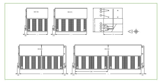
1. Drain ND50; 2. Outlet connection ND100; 3. Overflow ND80; Make up ND50 for VXI 144-x, 215-X, 288-X and ND80 for VXI 430-X; 5. Inlet connection ND100; 6. Vent ND15; 7. Access door.
